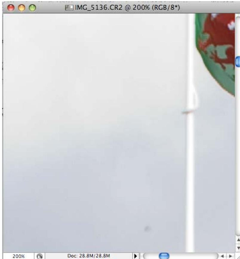
There is a small dust spec on the image and this can easily be removed. Select the **spot healing brush tool** and ensure the brush is large enough to cover the entire spot, click on the spot to remove the mark.
